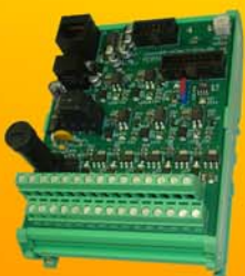
- NMEA expansion module (for VDR link) incl. software selector for stage #2 alarm - alarm transfer & emergency call facility (5 binary inputs & NMEA) NMEA 210.24.0.0
