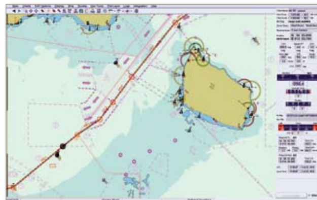
Route planning is done on ECDIS and NP 5000 ensures accurate track steering
