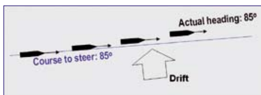
In Heading Control the course over ground line is affected by drift and wind
