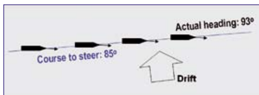
In Course Control the vessel stays on its course over ground line independently of drift and wind
